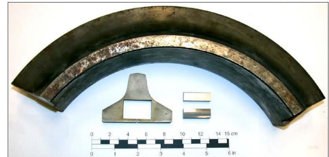
Part of a cutter ring, a 10 mm slice taken from the same ring, and two prepared AVS test pieces which are cut out of the centre of the slice.
