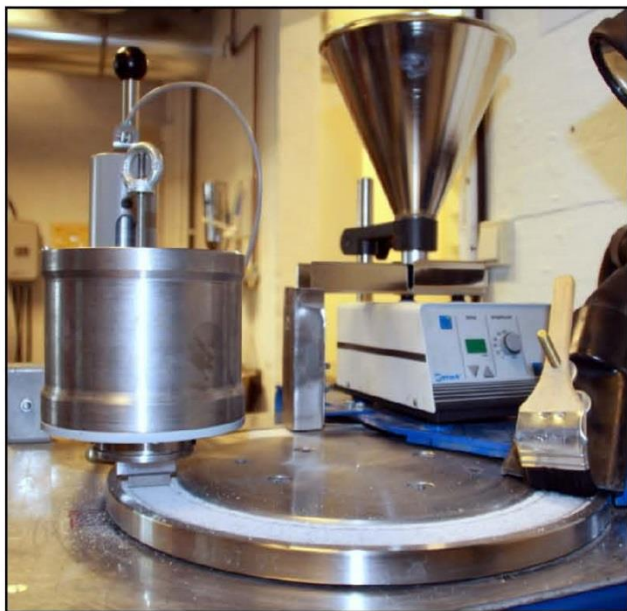
Test equipment used to determine Abrasion Value Cutter Steel (AVS) and Soil Abrasion Test (SAT™).
