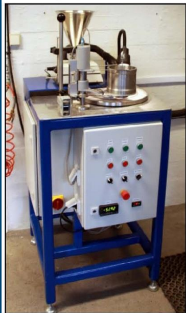
Test equipment used to determine Abrasion Value Cutter Steel (AVS) and Soil Abrasion Test (SAT™).
